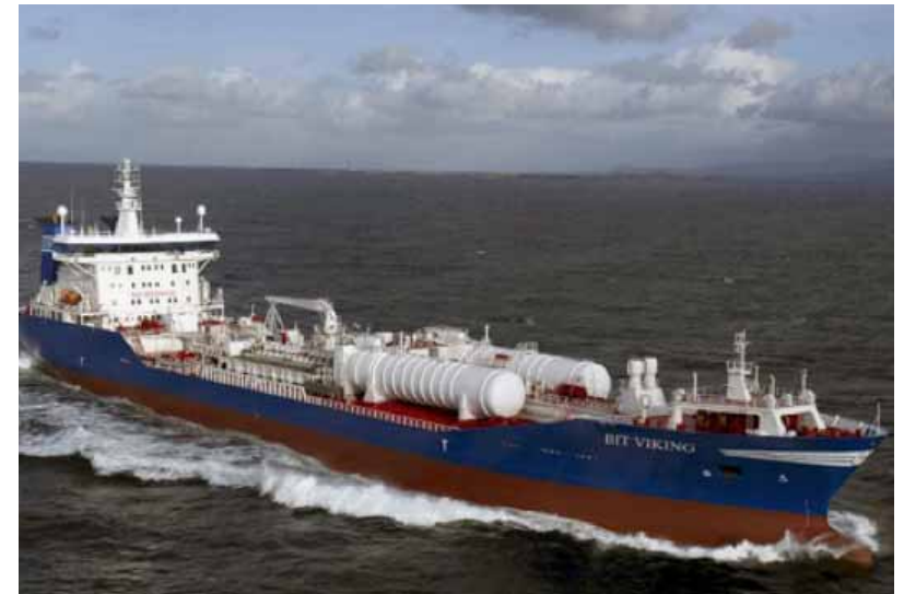
The Bit Viking utilises Wärtsilä's DF engines as well as a new LNGPac system, which enables the safe and convenient onboard storage of LNG.
