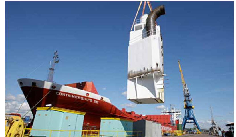
The Wärtsilä scrubber concept works with fresh water in a closed-loop system in which sulphur oxides are neutralised with caustic soda.
