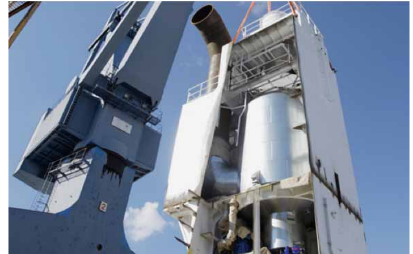
Wärtsilä has extensive experience from delivering SO x scrubbers for stationary power plants, and now also offers such solutions for ships.
